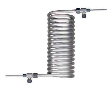
Dual Tube Coil (DTC) products are helically wound, full counter flow heat exchangers—well-suited for a variety of applications where low flow rates of high pressure and/or temperature fluids need heating or cooling. A variety of inner and outer tube sizes are available to meet most application requirements.
