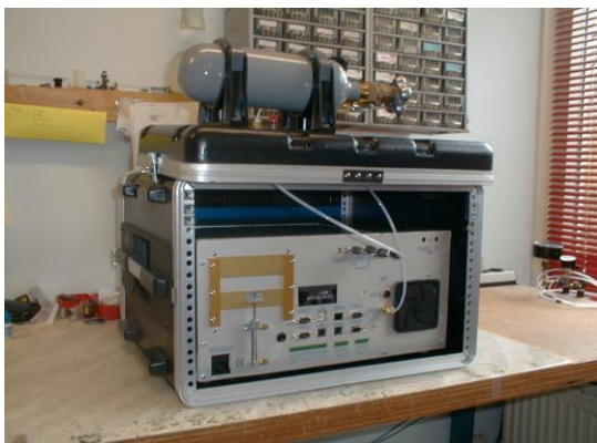
Mobile unit, can be run for several days on a 2 –l bottle of nitrogen, can be battery powered
